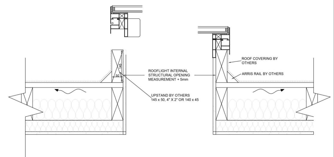
INTERNAL UPSTAND MEASUREMENTS ARE ROOFLIGHT INTERNAL MEASUREMENTS + 5mm
