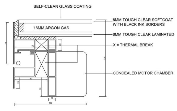
U-VALUE (THERMAL TRANSMITTANCE) OF 1.3 W/m<sup>2</sup>K TOTAL UNIT WEIGHT OF 45KG m<sup>2</sup>
